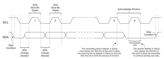
Figure 3-1. Start Condition, Data Transitions, Stop Condition, and Acknowledge
